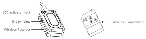
This mode will allow you to control the DB-60V using the wireless controller. It's including the transmitter and the receiver. You can control up to 4 independent machines, or many more if you run them simultaneously.
