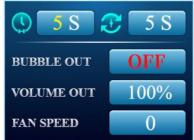
On this page, you can modify parameters by pressing <MENU>. The selected content will be highlighted in red, and you can change the current settings by pressing "A" and "V" button.
