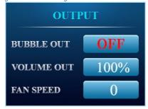
On this page, you can modify parameters by pressing <MENU>. The selected content will be highlighted in red, and you can change the current settings by pressing " $\blacktriangle$ " and " $\blacktriangledown$ " button.
