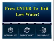
Low water level warning triggers when the water tank reaches the low-level threshold, water level exceeds minimum in the standby mode and the pump intake drops level below minimum in working mode.
