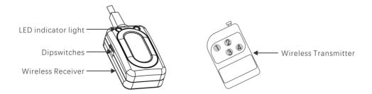
This mode will allow you to control the X-DB7 using the wireless controller. It includes the transmitter and the receiver. You can control up to 4 independent machines, or many more if you run them simultaneously. See the below instructions on setting up your operation with the wireless controller.
